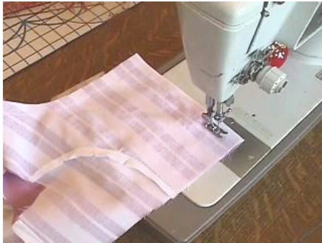
Bodice stitched to lining, leaving 5/8" free at bottom of back closure.
